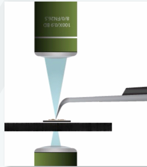
Extended transparent glass probe with high Q Factor
