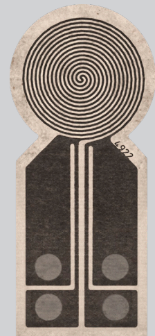
Mica-insulated Hot Disk ® sensors
