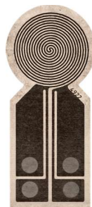
Mica-insulated Hot Disk® sensors Models 5465, 5082, 4921, 4922, and 5599.
