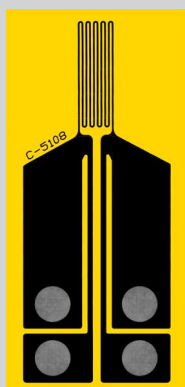
Kapton-insulated Hot Strip ® sensor
